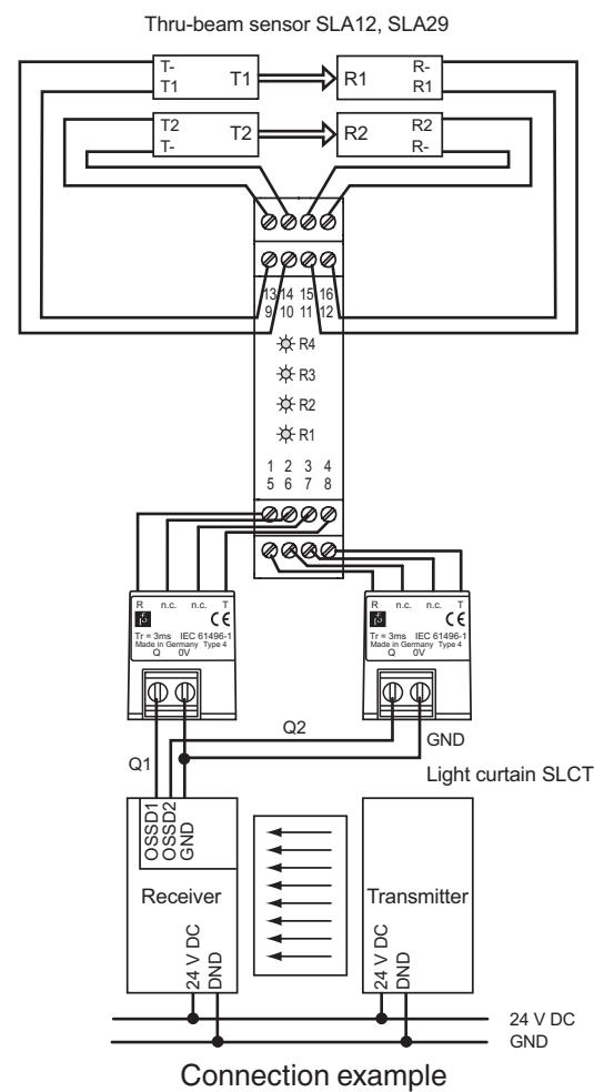
IF-SB4-01 is operated on a safety control interface unit type SafeBox SB4 on the modules SB4, 4CP, and 4C. Please note the operating instructions for the SafeBox.
