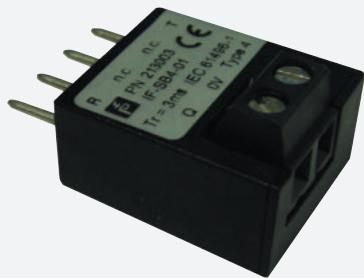
Interface for SafeBox SB4 modules 4CP and 4C
